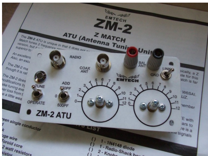
EMTECH ZM-2 Front panel Front panel completed with major components installed
