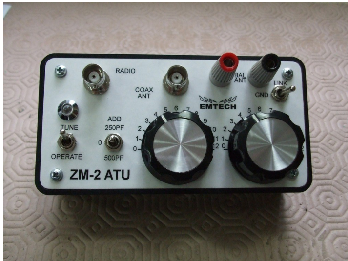
The ZM-2 Emtech Antenna Tuning Unit Complete build
