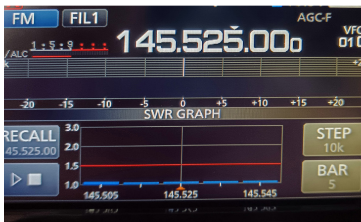
Showing near 1:1 SWR antenna match A near 1:1 SWR match
