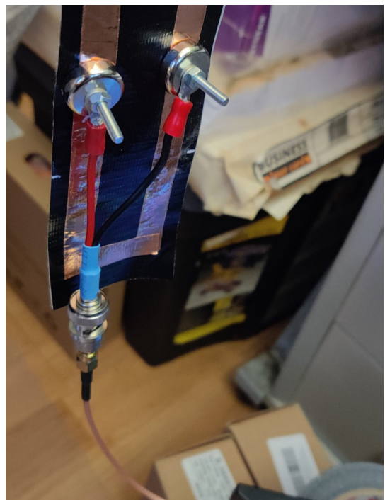
Testing the SWR with a nanoVNA
