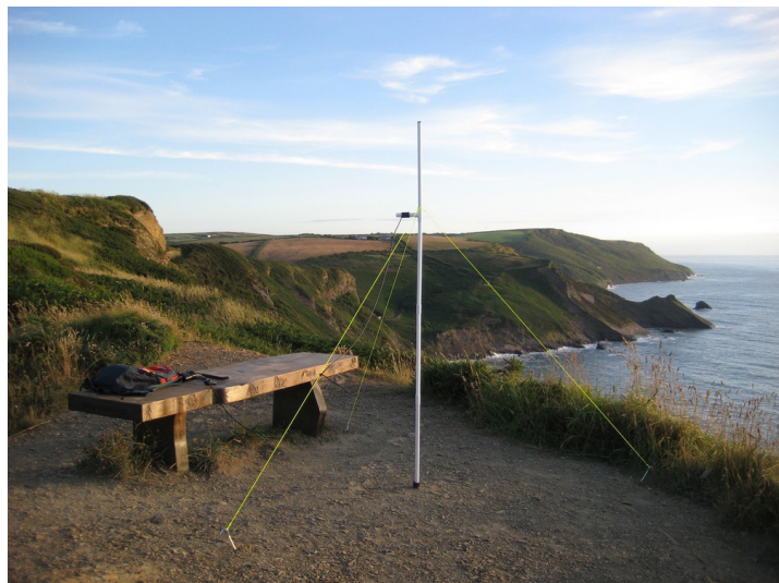
This photo shows my MFJ1621 Portable Antenna tuneable 7MHz (40M) to 10M (28 MHz).
